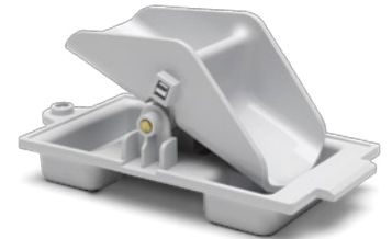
The ESP-SMT's tipping rain bucket measures rainfall, accounting for effective rainfall, in order to prevent under- or over-irrigation.
